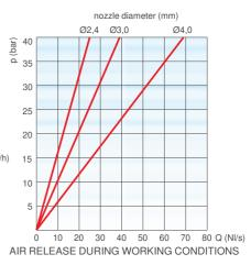
The air flow charts were created in Kg/s from laboratory tests and numerical analysis, without the screen, then converted in  $Nm^3/h$  using a safety factor.
